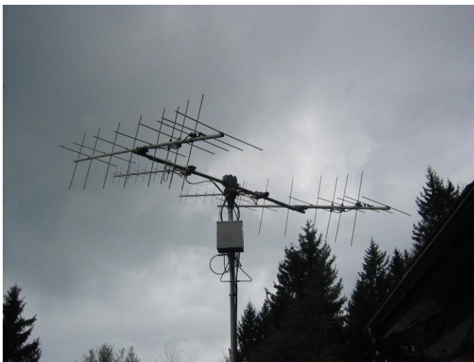
crossed Yagi accoppiate 144 (e 136) MHz - 430 MHz
